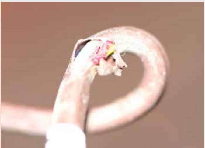
BARE METAL STAPLE: This staple is believed to have cut through this wire, causing the door to open when Parker handled it. (Photo used with permission.)
