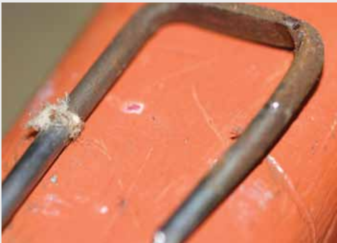
BARE METAL STAPLE: This staple is believed to have cut through this wire, causing the door to open when Parker handled it. (Photo used with permission.)
