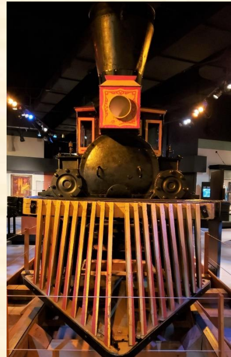
The cow-catcher on the 1848 Pioneer, Chicago's first locomotive, now at the Chicago History Museum
